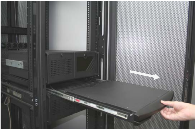
Figure 4. Pulling the tab toward the front of LCD.
